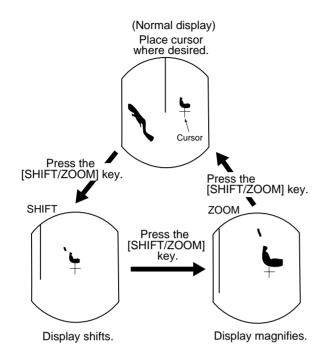
Figure 2-8 Shifting and zooming the display
